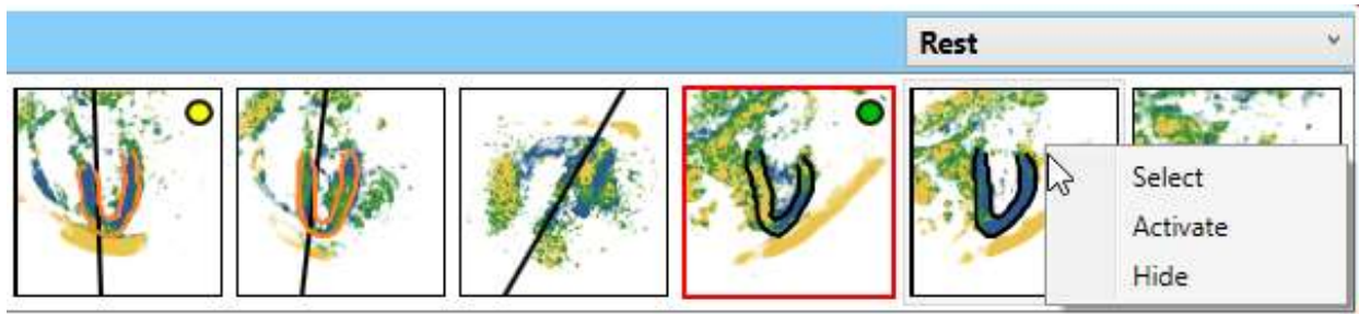
Figure 3-10: In the Image List, green radio buttons mark the slices being reported
